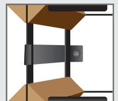
Stabilizer bracket secures rack against the wall.
